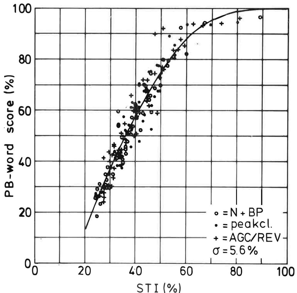
Figure 3. Relation between the objective STI and PB-word score for 167 different transmissior channels. The disturbances were combinations of bandpass limiting, noise, peak chipping, automatic gain control and reverberation.
