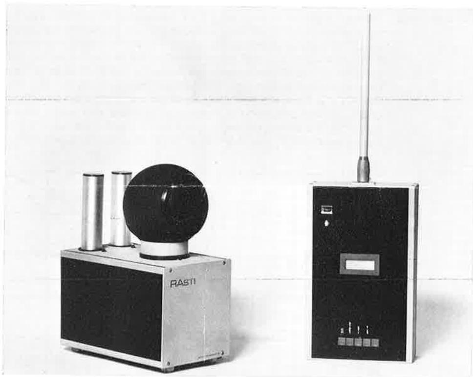
Figure 1. Signal source and analysis part of the measuring equipment RASTI.
