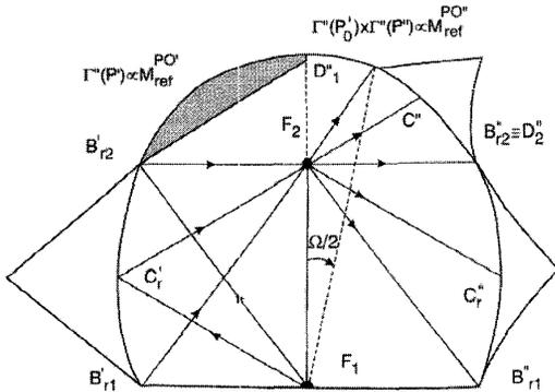
**Fig. 4** Paths of the doubly reflected rays, and profiles in the E-plane
