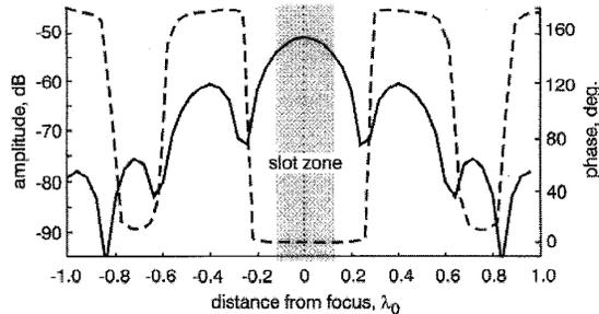
**Fig. 6** Amplitude and phase of the contribution  $|\vec{H}^{PO'} \cdot \hat{x}|$  along the minor axis of the ellipse (parallel to the slot)  $e = 0.5$ ,  $\epsilon_{r1} = 4$ , major semiaxis =  $5\lambda_0$ . The shadowed region corresponds to that occupied by the slot
