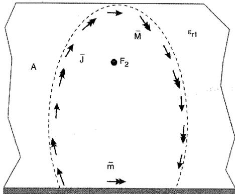
**Fig. 3** Equivalent currents at the lens interface
