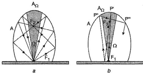
**Fig. 2** Reflection mechanisms inside the lens
