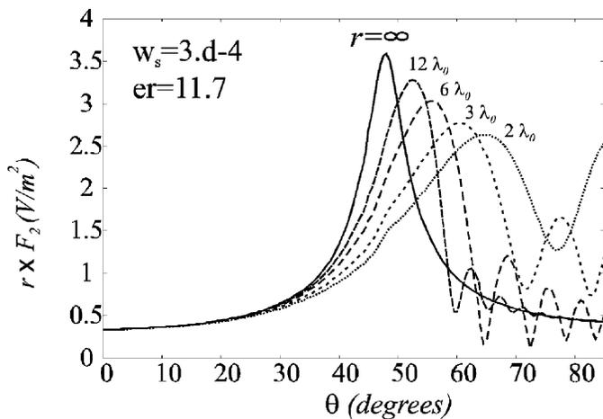
Fig. 9. Normalized electric potential ( $F_2$  multiplied by  $r$ ) from the near to far zone along radial angular scans at different distances ( $r = p\lambda_0, p = 1, 2, 3, 6, 12, \infty$ ). Slot and permittivities are the same as those in Fig. 3.
