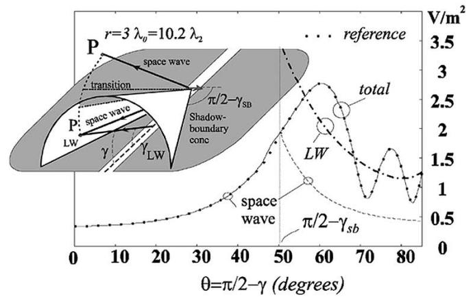
Fig. 8. Electric potential  $F_2$  in medium 2 at a distance  $r = 3\lambda_0$  as a function of the scan angle for a slot width  $w_s = 3 \cdot 10^{-4} \lambda_0$  and for permittivities  $\epsilon_{r1} = 1$  and  $\epsilon_{r2} = 11.7$ . The reference curve (dots) is almost superimposed to the uniform asymptotics (solid line) obtained by implementation of (35). Leaky wave (LW, dash-dotted line) and space wave (dashed line) are also presented.
