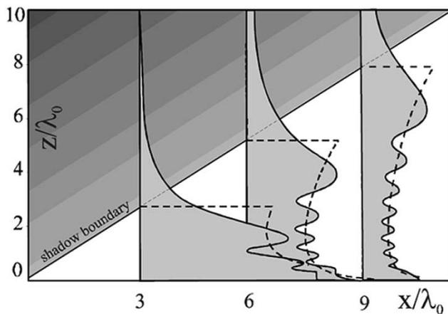
Fig. 10. Vertical scans of the amplitude of the field potential in medium 2 for  $y = 0$  and for  $x = 3\lambda_0, 6\lambda_0, 9\lambda_0$ . Dashed lines represent the exponentially growing (except for points very close to the slot) LW contribution.
