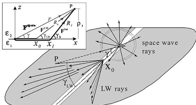
Fig. 1. Ray contributions in the denser medium. Space-wave ray propagate directly from the source with spherical spreading factor. Lateral- and leaky-wave ray arise from  $x_0$  and  $x_1$ , respectively, and next propagate toward  $P$  with the medium 2 wave speed. Both the leaky wave and the lateral wave have a conical wave-front (only the leaky wave is shown in the three-dimensional (3-D) view) with different spreading factor.
